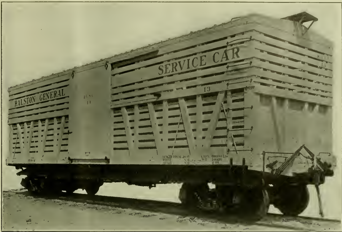
VIEW OF GENERAL SERVICE CAR WITH DROP DOORS RELEASED.
